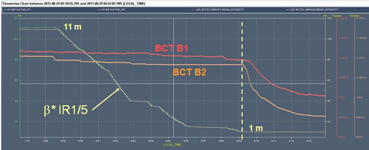
Figure 12: Evolution of the beam intensities during the high intensity test squeeze. A strong loss started exactly at the end of the squeeze to 1 m.
